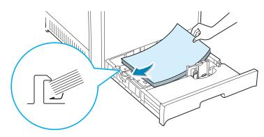
Make sure that all four corners are flat in the tray and under the corner brackets, as shown below.
